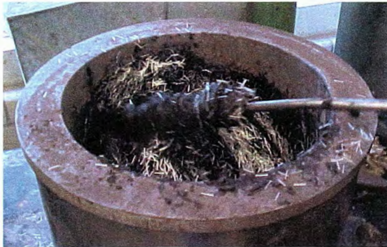
Figure 3.12 Melted composite material with fiberglass
