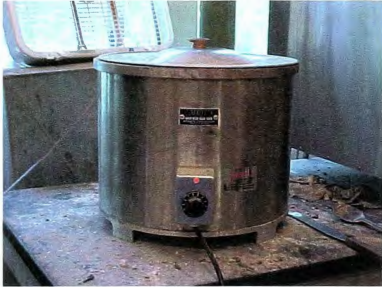
Figure 3.10 Electric melting pot used to melt PET
