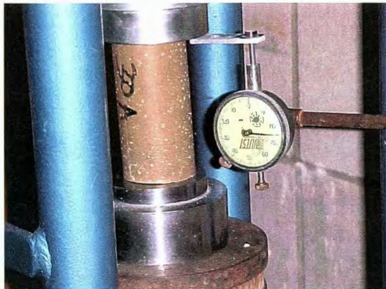
Figure 3.7 Compression test for cylinder specimens with vertical deformation measurements
