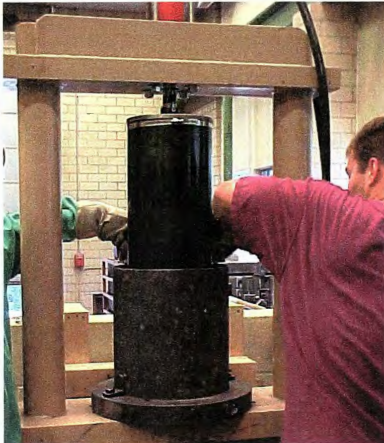
Figure 3.13 Centering the pipe with the wooden spacers
