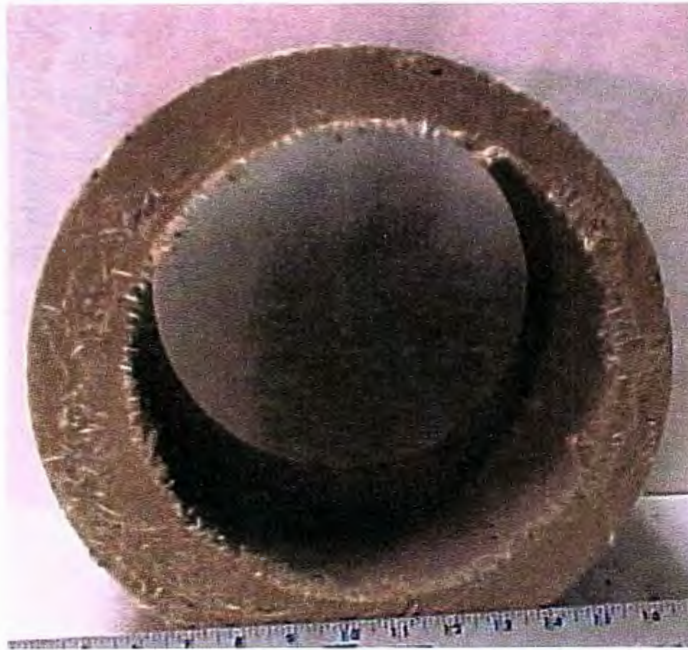
Figure 4.20 Pipe specimen #18 with 4% fiberglass content
