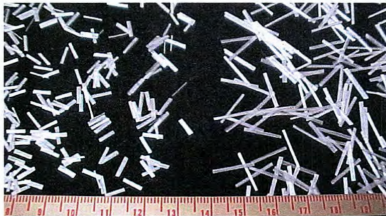
Figure 3.5 6 mm and 13 mm fiberglass fibers
