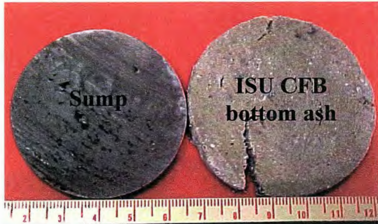
Figure 4.31 Water absorption test specimens
