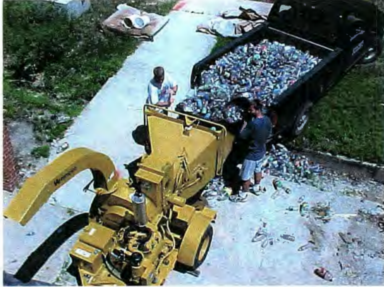
Figure 3.2 First stage in reducing the volume of PET from curbside recycling programs
