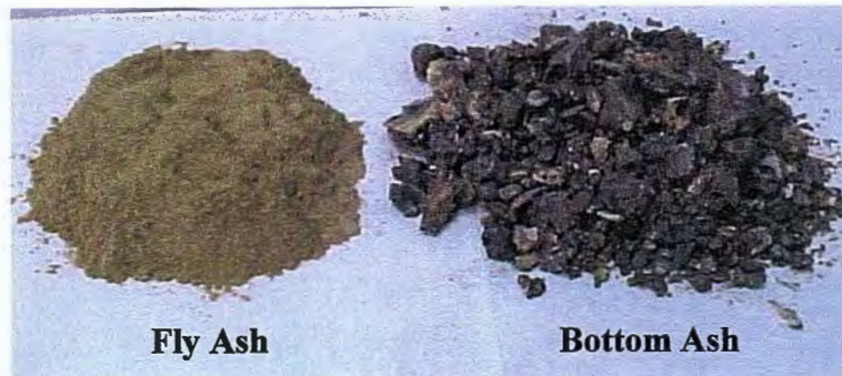
Figure 2.2 Ames fly ash and ISU CFB bottom ash (100 g shown)
